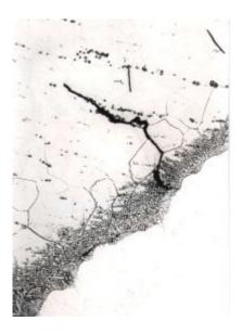
Similar to austenitic stainless steel, nickel alloys are susceptible to formation of liquation cracks in reheated weld metal regions or parent metal HAZ. This type of cracking is controlled by factors outside the control of the welder such as grain size or impurity content. Some alloys are more sensitive than others. For example, some cast superalloys are difficult to weld without inducing liquation cracks.
